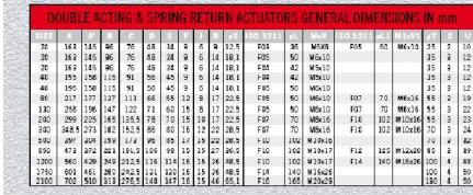
DOUBLE ACTING & SPRING RETURN ACTUATORS GENERAL DIMENSIONS IN mm
